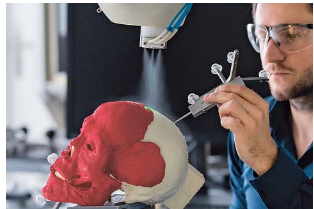
Precise and non-contact: CARLO cuts through bone with a laser beam.
